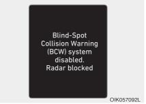
Blind-Spot Collision Warning (BCW) system disabled. Radar blocked
