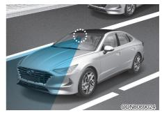
The front view camera is a sensor detecting the lane.
