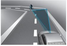
The front view camera or front radar sensor recognition system may not detect the vehicle, pedestrian or cyclist traveling in front on a curved road.
