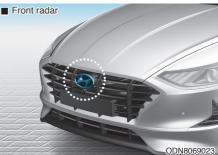
In order for FCA to operate properly, always make sure the sensor cover or sensor is clean and free of dirt, snow, and debris.
