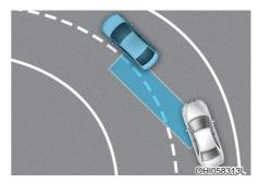
The system may not operate properly when driving on a curved road. In certain instances, the system may recognize a vehicle in the same lane.
