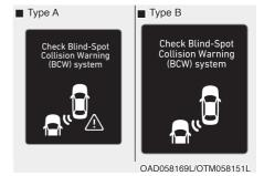
Check Blind-Spot Collision Warning (BCW) system
