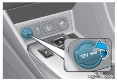
The power outlet is designed to provide power for mobile telephones or other devices designed to operate with vehicle electrical systems.
