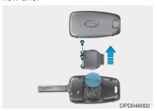
Battery Type: CR2032 To replace the battery:
