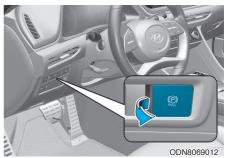
To apply the EPB (Electronic Parking Brake):
