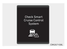
Check Smart Cruise Control System The message will appear when the vehicle distance control is not functioning normally.
