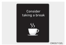
The "Consider taking a break" message appears on the cluster LCD display and a warning sounds to suggest that the driver take a break, when the driver's attention level is below 1.  DAW will not suggest a break, when the total driving time is shorter than 10 minutes and also does not recommend an additional break within 10 minutes after a break.
