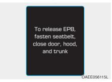
To release EPB, fasten seatbelt, close door, hood and trunk
