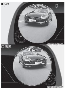
Blind-Spot View Monitor displays the left or right side of the rear blind spot area of your vehicle in the instrument cluster when the left or right turn signal is on. This function helps you drive safely when changing lanes.
