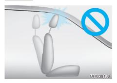
If you recline the seatback towards the front with the head restraint and seat cushion raised, the head restraint may come in contact with the sunvisor or other parts of the vehicle.
