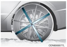
Since the sidewalls of radial tires are thinner than other types of tires, they may be damaged by mounting some types of tire chains on them. Therefore, the use of snow tires is recommended instead of tire chains. Do not mount tire chains on vehicles equipped with aluminum wheels; if unavoidable use a wire type chain.
