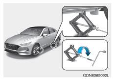
Insert the jack handle into the jack and turn it clockwise, raising the vehicle until the tire clears the ground. Make sure the vehicle is stable on the jack.
