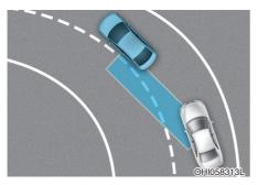
BCW and BCA may not operate properly when driving on a curved road. In certain instances, the system may recognize a vehicle in the same lane.
