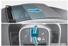
If you pull the sunroof control lever (1) backward, the sunshade will slide all the way open then the sunroof glass will slide all the way open. To stop the sunroof movement at any point, pull or push the sunroof control lever (1) momentarily.
