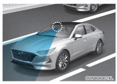
Lane Following Assist helps detect lane markers on the road with a front view camera at the front windshield. and assists the driver's steering to help keep the vehicle between lanes.
