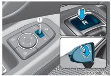
When you press the R (Reverse) button, the outside rearview mirror(s) will rotate downwards to aid with driving in reverse.
