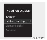
To activate the head up display, select 'Enable Head-Up Display' on the User Settings mode on the instrument cluster LCD display.
