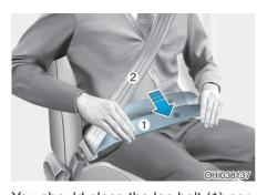
You should place the lap belt (1) portion across your hips and the shoulder belt (2) portion across your chest. The seat belt automatically adjusts to the proper length after the lap belt portion is adjusted manually so that it fits snugly around your hips. If you lean forward in a slow, easy motion, the belt will extend and move with you.
