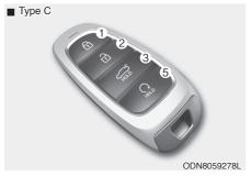
Your HYUNDAI uses a Smart Key, which you can use to lock or unlock a door (and trunk) and even start the engine.
