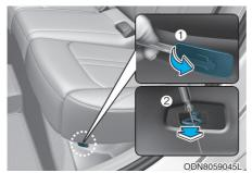
Open the cable cover(1) under the rear seat with a mechanical key and pull the cable (2) for unlocking the trunk. The cable is fixed firmly so it may hard to pull. Therefore, please put auxiliary equipment such as a screwdriver to the loop and pull it comfortably.
