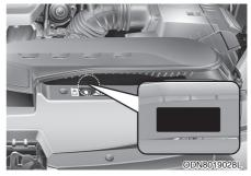
Your vehicle is filled with R-134a or R-1234yf according to the regulation in your country at the time of production. You can find out which air conditioning refrigerant is applied to your vehicle on the label located in front of the engine compartment.
