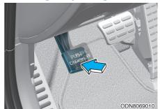
Check whether the stroke is within specification when the parking brake pedal is depressed with 20 kg (44 lb, 196N) of force. Also, the parking brake alone should securely hold the vehicle on a fairly steep grade. If the stroke is more or less than specified, we recommend that the system be serviced by an authorized HYUNDAI dealer.
