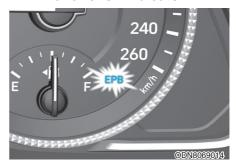
If the EPB malfunction indicator remains on, comes on while driving, or does not come on when the ignition switch is changed to the ON position, this indicates that the EPB may have malfunctioned.
