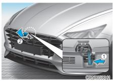
3. Go to the front of the vehicle, raise the hood slightly, push the secondary latch up (1) inside of the hood center and lift the hood (2). After it has been raised about halfway, it will raise completely by itself.
