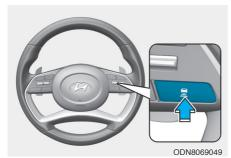
When Smart Cruise Control is ON, you can set and maintain the distance from the vehicle ahead of you without pressing the accelerator or brake pedal.
