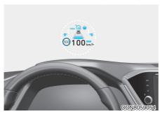
The head up display is a transparent display which projects a shadow of some information of the instrument cluster and navigation on the display located on the windshield glass.
