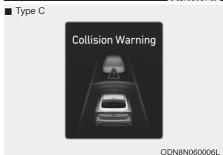
This warning message appears on the LCD display with a warning chime. Additionally, some vehicle system intervention occurs by the engine management system to help decelerate the vehicle.
