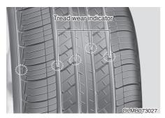
If the tire is worn evenly, a tread wear indicator will appear as a solid band across the tread. This shows there is less than 1.6 mm (1/16 in.) of tread left on the tire. Replace the tire when this happens.
