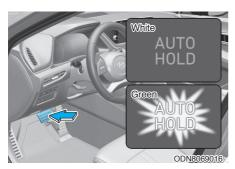
When you stop the vehicle completely by depressing the brake pedal, the AUTO HOLD indicator changes from white to green.
