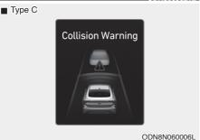
This warning message appears on the LCD display with a warning chime.
