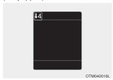
In the manual shift mode, this indicator informs which gear is desired while driving to save fuel.
