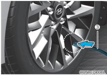
Unscrew the valve cap from the valve of the defective wheel and screw the filling hose (3) of the sealant bottle onto the valve.
