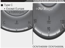
This gauge indicates the temperature of the engine coolant when the ignition switch is in the ON position.
