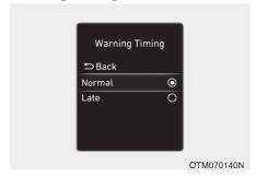
The driver can select the initial warning activation time on the LCD display or infotainment system display.
