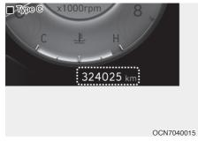
The odometer indicates the total distance that the vehicle has been driven and should be used to determine when periodic maintenance should be performed.
