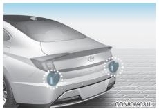
The rear corner radars are the sensors inside the rear bumper for detecting the side and rear areas. Always keep the rear bumper clean for proper operation of the system.
