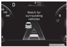
If the vehicle ahead (vehicle speed: less than 30km/h) disappears to the next lane, the warning chime will sound and a message "Watch for surrounding vehicles" will appear. Adjust your vehicle speed for vehicles or objects that can suddenly appear in front of you by depressing the brake pedal.
