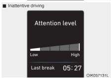
The driver can monitor his/her driving conditions on the cluster LCD display. The DAW screen will appear when you select the Assist mode tab ( ) on the LCD display if the system is activated. For more details, refer to "LCD Display Modes" in chapter 4.
