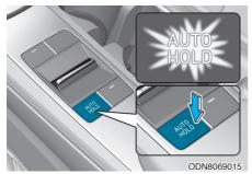
With the driver's door, engine hood and trunk closed, depress the brake pedal and then press the [AUTO HOLD] switch. The white AUTO HOLD indicator will come on and the system will be in the standby position.
