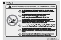
Never install a child restraint in the front passenger's seat. An inflating air bag can forcefully strike a child or restraint resulting in serious or fatal injury.
