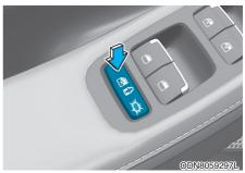
If you push the Electronic child safety lock button and the indicator illuminates, rear passengers can not open the rear door from inside the vehicle. To cancel the Electronic child safety lock system, you push the Electronic child safety lock system button one more time and then the indicator turns off.
