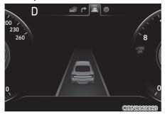
To see the LKA screen on the LCD display in the cluster, select Driving Assist mode (A). For more details, refer to "LCD Display Modes" in chapter 4.
