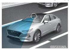
Lane Keeping Assist with a camera at the front windshield, helps detect lane markers on the road, and assists the driver's steering to help keep the vehicle between lanes.
