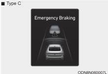
This warning message appears on the LCD display with a warning chime. Additionally, some vehicle system intervention occurs by the engine management system to help decelerate the vehicle.
