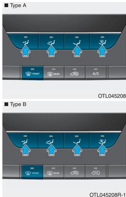
The mode selection button controls the direction of the air flow through the ventilation system.
