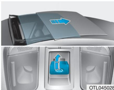
If you pull the sunroof control lever backward, the sunshade will slide all the way open then the sunroof glass will slide all the way open. To stop the sunroof movement at any point, pull or push the sunroof control lever momentarily.
