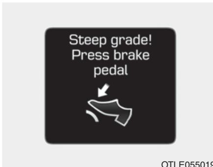
This warning message is displayed when vehicle is driven slowly on a grade and the vehicle detects that the brake pedal is not applied.
