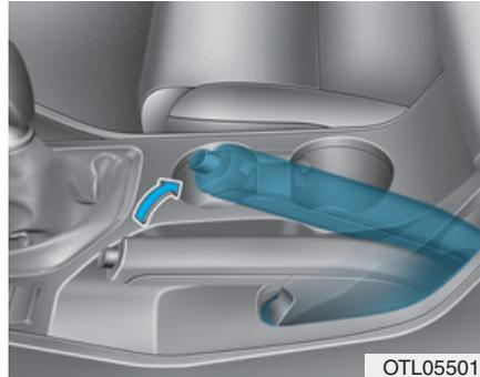
Check the stroke of the parking brake by counting the number of “clicks” heard while fully applying it from the released position. Also, the parking brake alone should securely hold the vehicle on a fairly steep grade. If the stroke is more or less than specified, we recommend that the system be serviced by an authorized HYUNDAI dealer.
