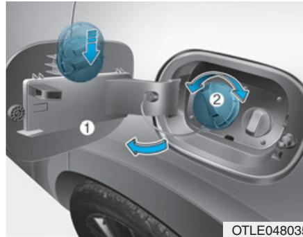
4. Pull the fuel filler door (1) out to fully open.
