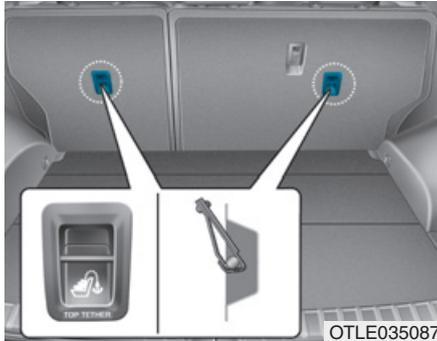
Child Restraint hook holders are located on the rear of the seatbacks.
