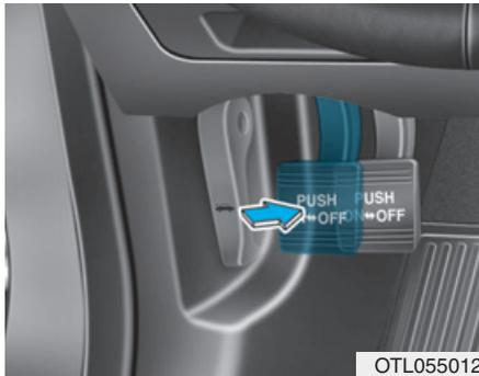
Check whether the stroke is within specification when the parking brake pedal is depressed with 20 kg (44 lb, 196N) of force. Also, the parking brake alone should securely hold the vehicle on a fairly steep grade. If the stroke is more or less than specified, we recommend that the system be serviced by an authorized HYUNDAI dealer.
