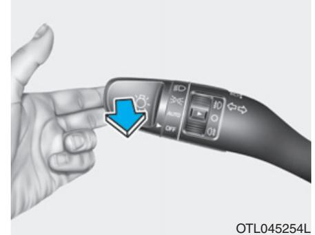
To flash the high beam headlamp, pull the lever towards you, then release the lever. The high beams will remain ON as long as you hold the lever towards you.
