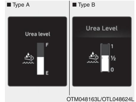
The urea solution gauge indicates the approximate amount of remaining urea solution inside the urea solution tank.
