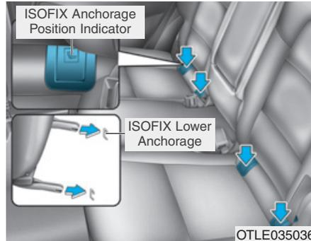
The ISOFIX anchorages symbols are located on the left and right rear seat cushions to identify the position of the ISOFIX anchorages in your vehicle (see arrows in illustration).
