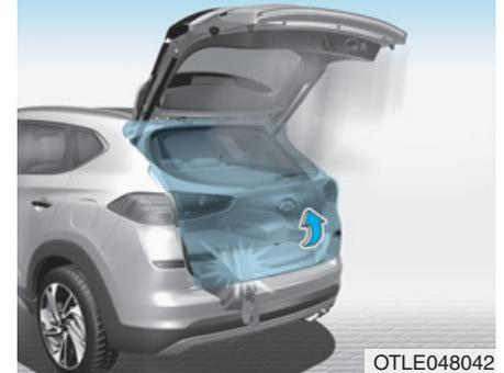
During power opening and closing if the power tailgate is blocked by an object or part of the body, the power tailgate will detect the resistance.
