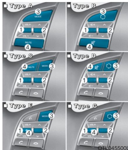
The audio control buttons on the steering wheel are provided for your convenient audio control, while safely driving.
