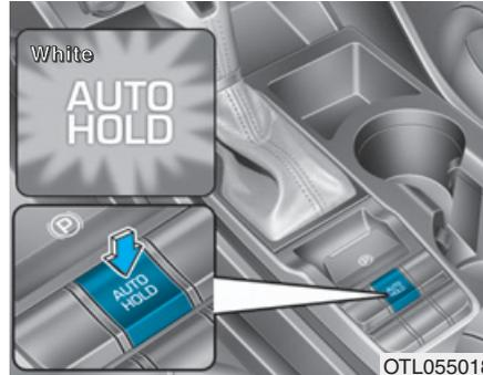
1. With the driver's door, engine hood and tailgate closed, fasten the driver's seat belt or depress the brake pedal and then press the [AUTO HOLD] switch. The white AUTO HOLD indicator will come on and the system will be in the standby position.
