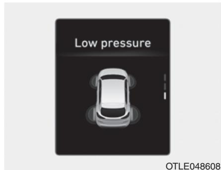
This warning message illuminates if the tire pressure is low with the Engine Start/Stop button in ON position.
