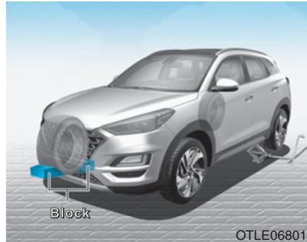
5. Block both the front and rear of the tire diagonally opposite of the tire you are changing.
