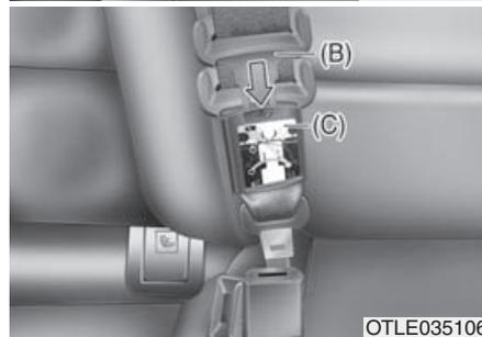
2. Insert the tongue plate (B) into the pocket (C)
