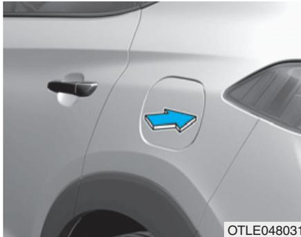
3. To open the fuel filler door, press the center edge of the fuel filler door.
