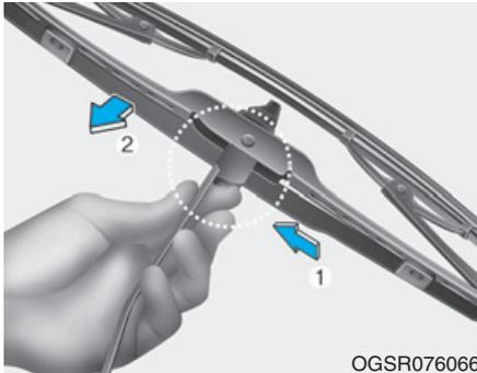
1. Lift up the wiper blade clip. Then lift up the wiper blade.
