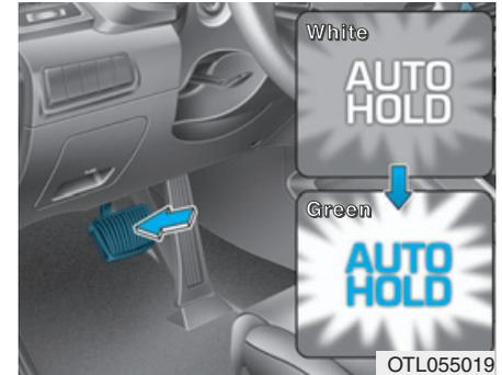
2. When you stop the vehicle completely by depressing the brake pedal, the AUTO HOLD indicator changes from white to green.
