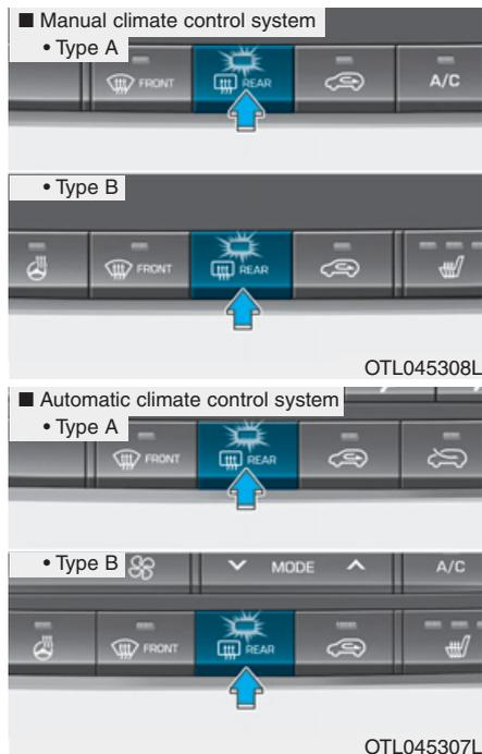
The defroster heats the window to remove frost, fog and thin ice from the interior and exterior of the rear window, while engine is running.
