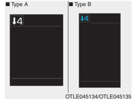
In the Sports Mode, this indicator informs which gear is desired while driving to save fuel.
