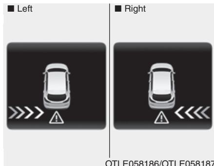
If the vehicle detected by the sensors approaches your vehicle, the warning chime will sound, the warning light on the outside rearview mirror will blink and a message will appear on the LCD display.
