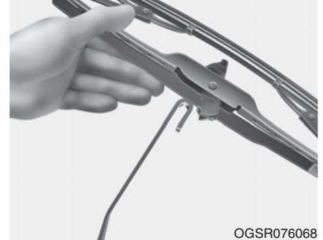
3. Remove the wiper blade from the wiper arm.
