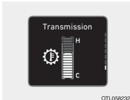
This mode displays the temperature of dual clutch transmission.
