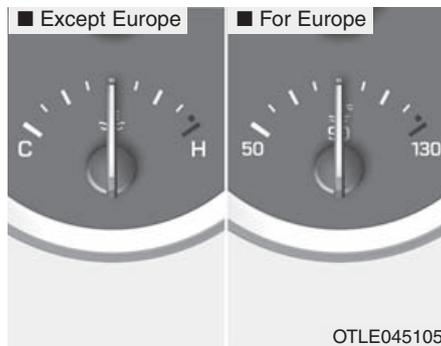
This gauge indicates the temperature of the engine coolant when the ignition switch or Engine Start/Stop button is in the ON position.
