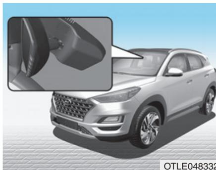
Auto defogging reduces the possibility of fogging up the inside of the windshield by automatically sensing the moisture of inside the windshield. The auto defogging system operates when the heater or air conditioning is on.
