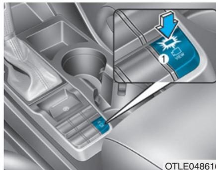
The Surround View Monitor system can assist in parking by allowing the driver to see around the vehicle.
