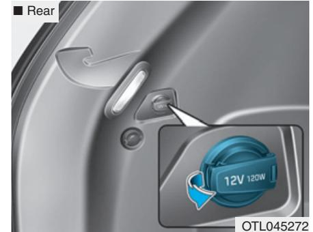
The power outlet is designed to provide power for mobile telephones or other devices designed to operate with vehicle electrical systems.
