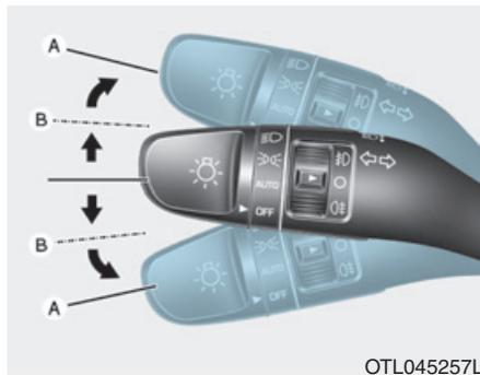
To signal a turn, push down on the lever for a left turn or up for a right turn in position (A). To signal a lane change, move the turn signal lever slightly and hold it in position (B).
