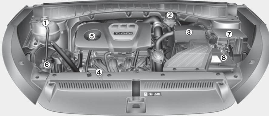
1. Engine coolant reservoir/Radiator cap
