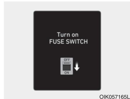
This warning message illuminates if the fuse switch located on the fuse box under the steering wheel is OFF. It means that you should turn the fuse switch on.
