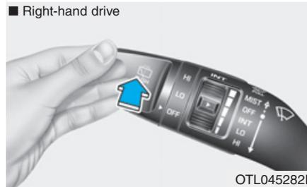
Push the lever away from you to spray rear washer fluid and to run the rear wipers 1~3 cycles. The spray and wiper operation will continue until you release the lever. (if equipped)
