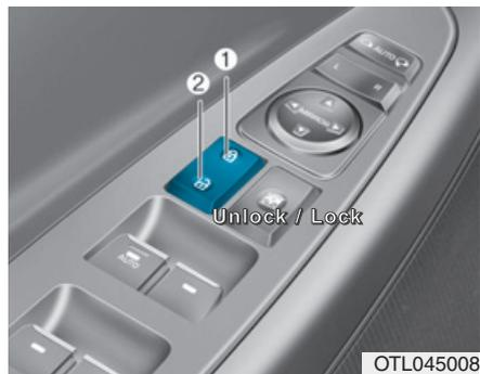
When pressing the (🔒) portion (1) of the switch, all vehicle doors will lock.
