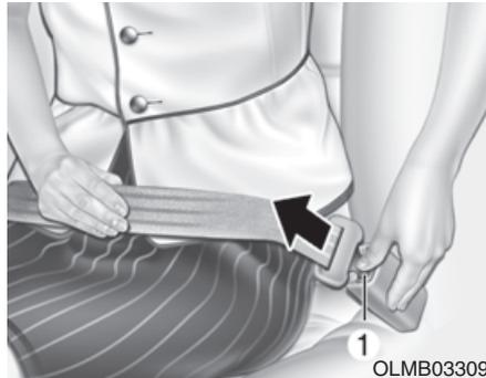
To release the rear center seat belt: Press the release button (1) on the buckle and remove the metal tab from the buckle.
