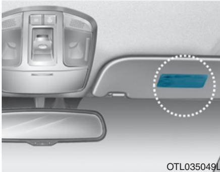
Air bag warning labels are attached to alert the passengers of potential risks of the air bag system.
