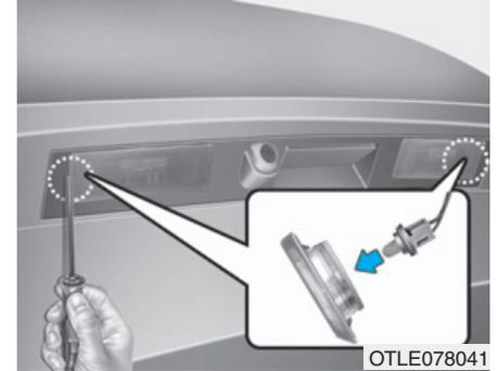
1. Loosen the lens retaining screws with a screwdriver.
