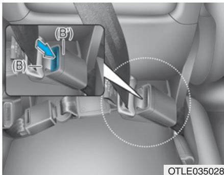
4. Pull the tongue plate (B) and insert it into the buckle (B') until an audible “click” is heard, indicating the latch is locked. Make sure the belt is not twisted.
