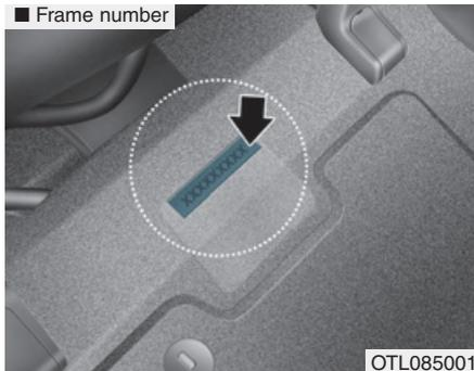
The vehicle identification number (VIN) is the number used in registering your vehicle and in all legal matters pertaining to its ownership, etc. The number is punched on the floor under the passenger seat. To check the number, open the cover.
