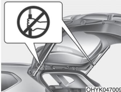
Do not hold the part (gas lifter) that supports the tailgate. Be aware that the deformation of the part may cause vehicle damage and a risk of safety accident.
