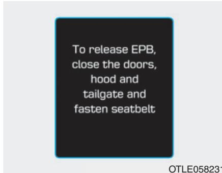
To release EPB, close the doors, hood and tailgate and fasten seatbelt
