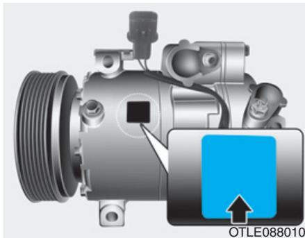
A compressor label informs you the type of compressor your vehicle is equipped with such as model, supplier part number, production number, refrigerant and refrigerant oil.
