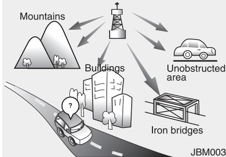
FM broadcasts are transmitted at high frequencies and do not bend to follow the earth's surface. Because of this, FM broadcasts generally begin to fade within short distances from the station. Also, FM signals are easily affected by buildings, mountains, and obstructions. This can lead to undesirable or unpleasant listening conditions which might lead you to believe a problem exists with your radio. The following conditions are normal and do not indicate radio trouble :
