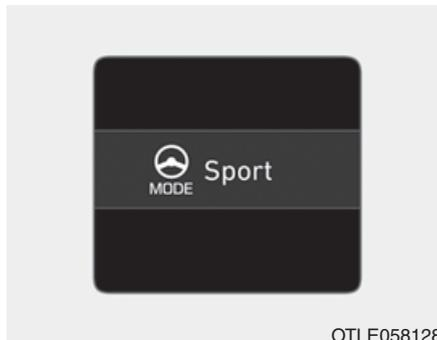
The sport steering mode offers high steering effort, making the wheel steering heavier. The sport steering mode is often used for driving on a highway.
