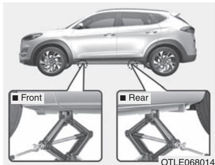
7. Place the jack at the designated jacking position under the frame closest to the tire you are changing. The jacking positions are plates welded to the frame with two notches and two dimples. Never jack any other position or part of the vehicle. It may damage to the side seal molding.
