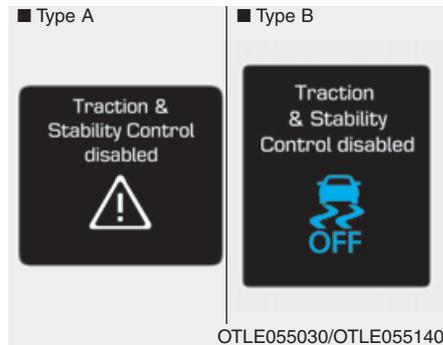
Press the ESC OFF button for more than 3 seconds. ESC OFF indicator light and message illuminates and ESC OFF warning chime will sound. At this state, the engine control function and brake control function does not operate. The vehicle stability control function does not operate any more.
