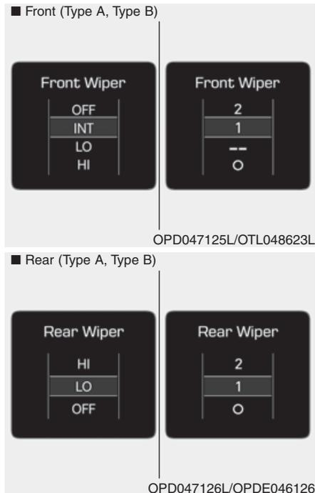
This indicator displays which wiper speed is selected using the wiper control.
