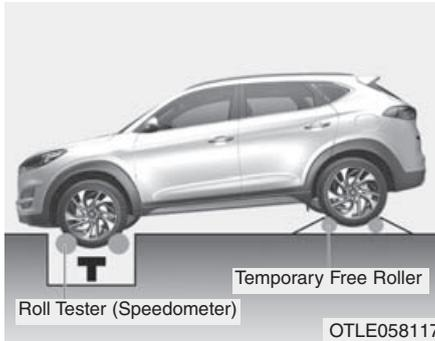
A full-time 4WD vehicle should not be tested on a 2WD roll tester. If a 2WD roll tester must be used, perform the following procedure:
