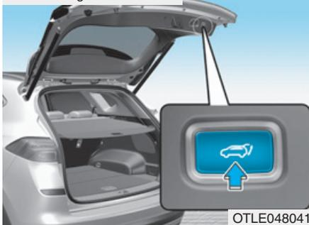
To activate or de-activate the power tailgate, go to User Settings mode and select the Power Tailgate on the LCD display.
