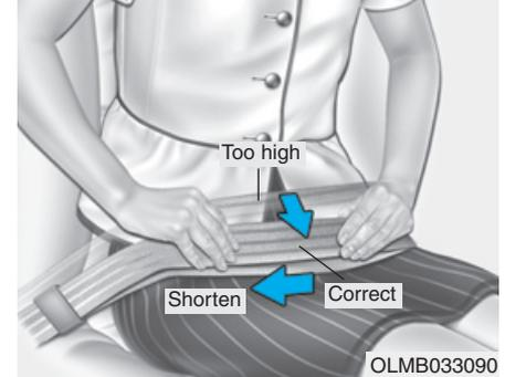
The length must be adjusted manually so it fits snugly around your hip. Fasten the belt and pull the loose end to tighten the belt.
