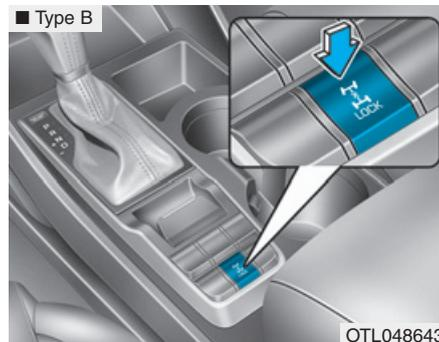
The Four Wheel Drive (4WD) System delivers engine power to all front and rear wheels for maximum traction.
