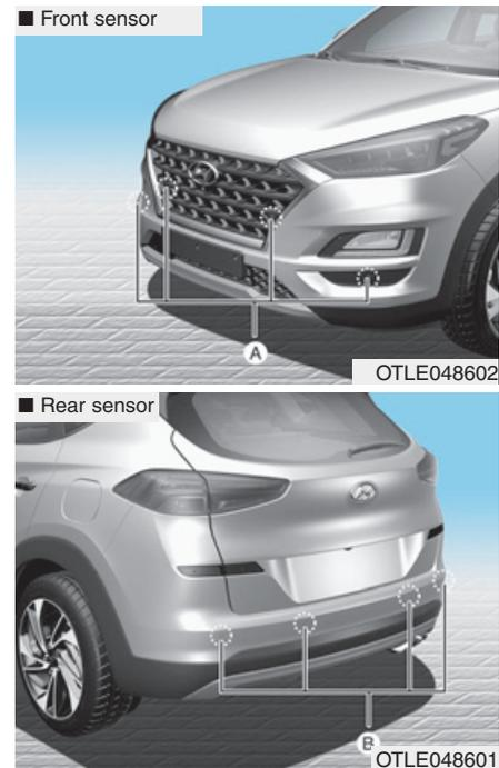
[A] : Front sensor, [B] : Rear sensor
