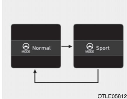
The steering mode options appear on the LCD display, when the driver presses the steering mode button.
