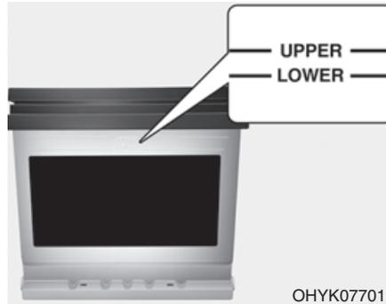
If your vehicle is equipped with a battery marked with LOWER (MIN) and UPPER (MAX) on the side, you should check the electrolyte level.
