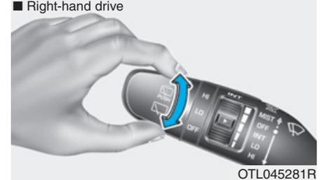
The rear window wiper and washer switch is located at the end of the wiper and washer switch lever. Turn the switch to the desired position to operate the rear wiper and washer.
