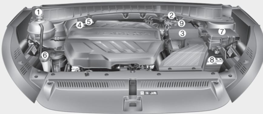
1. Engine coolant reservoir/Radiator cap
