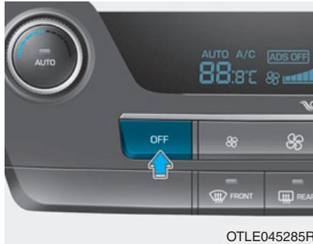
Push the OFF button of the front to turn off the air climate control system. However, you can still operate the mode and air intake buttons as long as the ignition switch is in the ON position.
