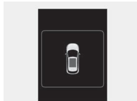
If the driver removes the ignition key (Smart key : turns off the engine) and opens the driver-side door when the sunroof is not fully closed, the warning chime will sound for approximately 3 seconds and sunroof open image will appear on the LCD display.
