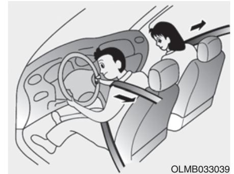
Your vehicle is equipped with driver's and front passenger's Pre-tensioner Seat Belts. The purpose of the pre-tensioner is to make sure the seat belts fit tightly against the occupant's body in certain frontal collisions. The pre-tensioner seat belts may be activated in crashes where the frontal collision is severe enough, together with the air bags.
