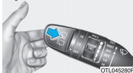
In the OFF (O) position, pull the lever gently toward you to spray washer fluid on the windshield and to run the wipers 1-3 cycles. The spray and wiper operation will continue until you release the lever.
