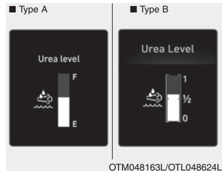
This mode displays the amount of the remaining urea solution in the urea solution tank.
