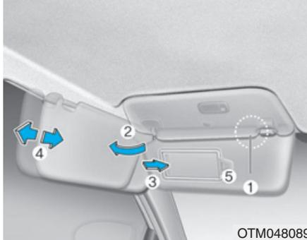
To use a sunvisor, pull it downward. To use a sunvisor for a side window, pull it downward, unsnap it from the bracket (1) and swing it to the side (2). To use the vanity mirror, pull down the sunvisor and slide the mirror cover (3). Adjust the sunvisor forward or backward (4) as needed. Use the ticket holder (5) to hold tickets.
