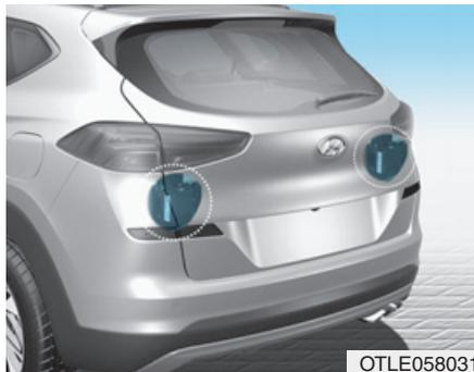
The sensors are located inside the rear bumper.
