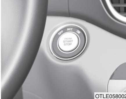
Whenever the front door is opened, the Engine Start/Stop button will illuminate and will go off 30 seconds after the door is closed. (if equipped)
