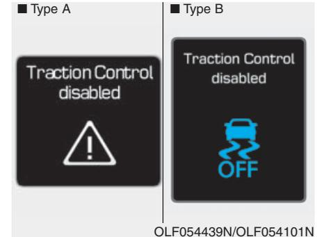
Press the ESC OFF button shortly (ESC OFF indicator light and message illuminates). At this state, the engine control function does not operate. The traction control function does not operate but only the brake control function operates.
